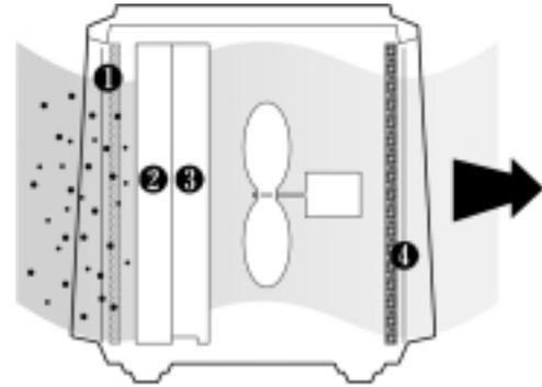
1. The PRE-FILTER catches the larger particles as room air is drawn through the rear grille.
