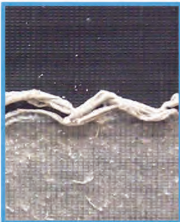
PreVent Wrap-Around filter 6 days after installation during cottonwood season.
